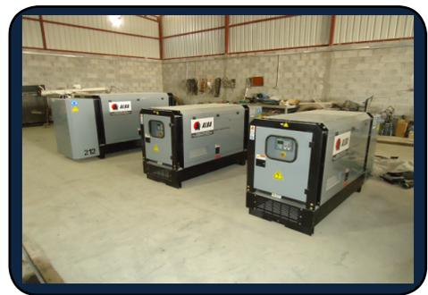
20 kva diesel generator set with super sound attenuated canopy
